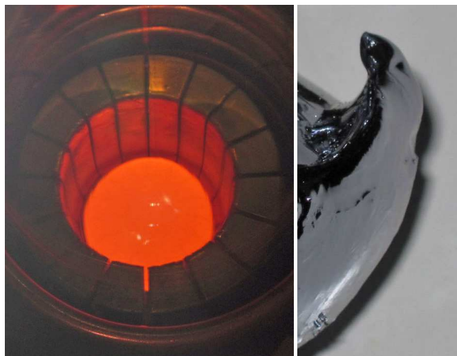
Fig. 4. Cold crucible melt and solidified, last-to-freeze region
