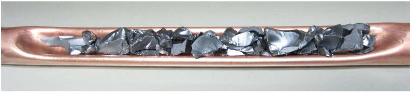
Fig. 7 Copper cold boat with typical 30g polysilicon chip and chunk charge
