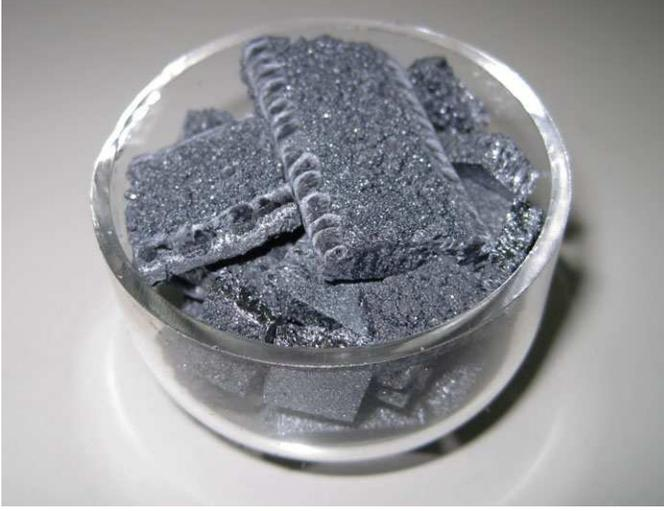
Fig. 3. APIVT polysilicon slabs in a quartz crucible for CZ growth
