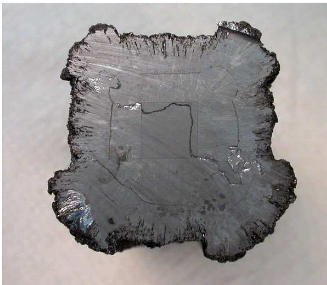
Fig. 7. Cross-section of 2<sup>nd</sup> APIVT polysilicon sample
